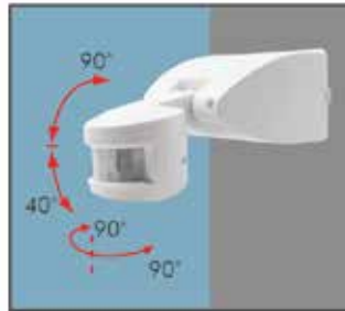
Detector head is adjustable 90° up & 40° down, and 90° left & 90° right
